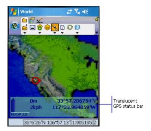
The background color of the GPS Status Bar indicates the current conditions of the GPS measurements according to the alerts that have been defined in ArcPad. A GREEN background indicates that the quality is acceptable according to the set alerts (alerts are set in the GPS properties dialog), YELLOW indicates that the quality parameters are not met, and RED indicates no fix.
