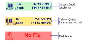
The GPS Status Bar also shows current position, current speed and altitude (if applicable).
